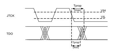
Figure 14: JTAG Interface Input AC Timing Diagram
